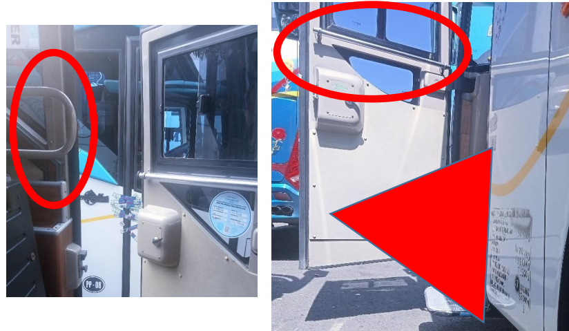
Figure 6. View of a stanchion in the bus (left [red circle]) and Handrail on the Bus (right), it appears that the handrail (red circle) is not in the same direction as the stair pathway (arrow). (Resources: personal documentation of author, 2023)
